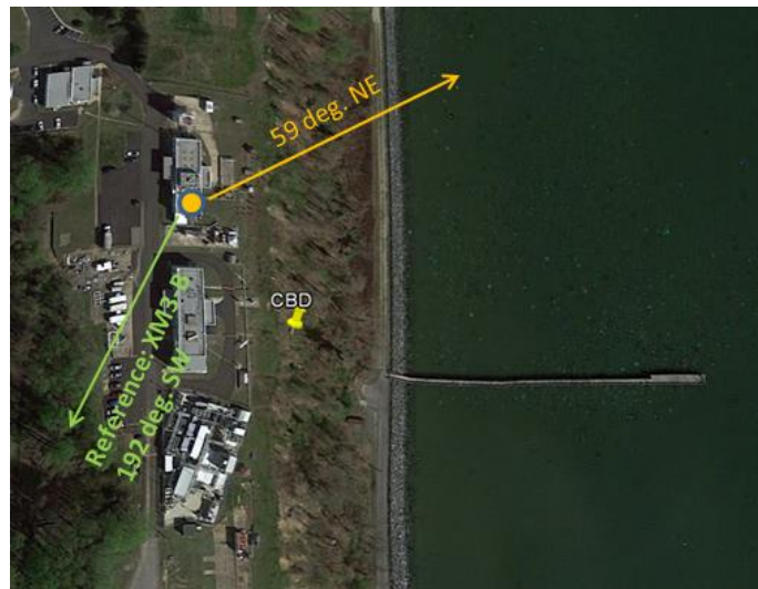
Figure 5-6: Top-down view of the bistatic geometry employed to image ship traffic at NRL-CBD using the BISCUIT 2.0 system. The yellow dot represents the physical location of the receiver and the reference / surveillance antennas. The green arrow shows the azimuth pointing direction of the reference antenna, while the yellow arrows shows the azimuth pointing direction of the surveillance antenna.
