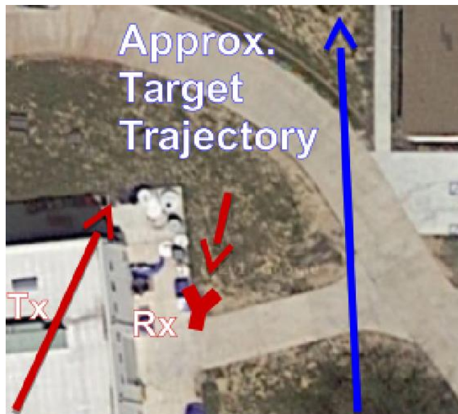
Figure 5-4: A top-down illustration of the measurement geometry for passive radar detection of aerial vehicles at the NRL-DC LASR facility.
