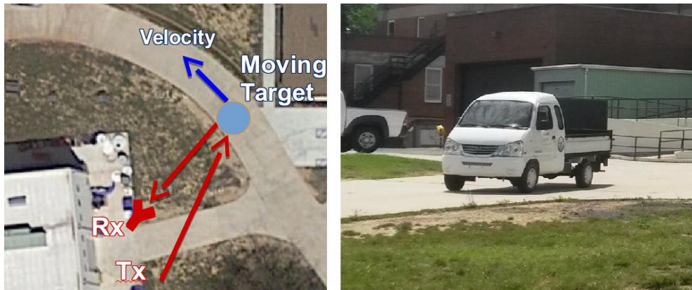
Figure 5-1: (Left) A top-down illustration of the measurement geometry for passive radar detection of ground vehicles at NRL-DC. (Right) A picture of the golf cart whose bistatic Doppler response is shown in Figure 5-2.
